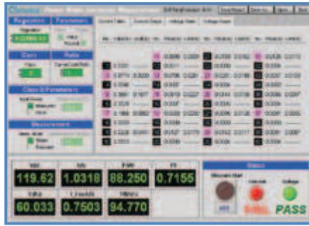
IEC 61000-3-2 Current Harmonics Test (Pre-compliance)
